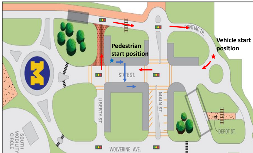
Figure 3.7: Urban portion of Mcity test track used for the study. The red star indicated the vehicle starting position, hidden from the pedestrian’s sight initially. The blue star indicates the starting position of the pedestrian. The red and blue arrows indicate the paths followed by the vehicle and the pedestrian respectively for one interaction.
