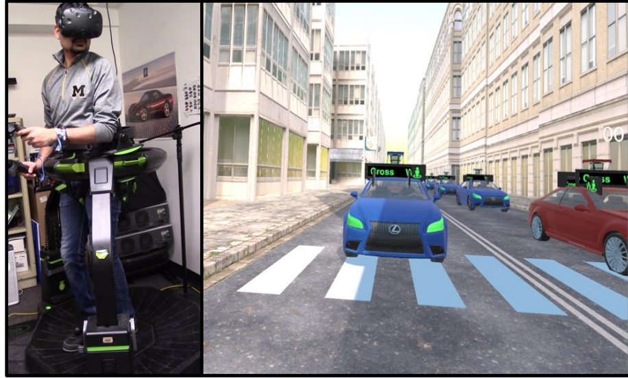
Figure 3.2: Virtual Reality setup for user study. The left side shows the user wearing the HTC Vive headset and walking on the omni-directional treadmill. The right side shows the virtual environment as seen by the participant.
