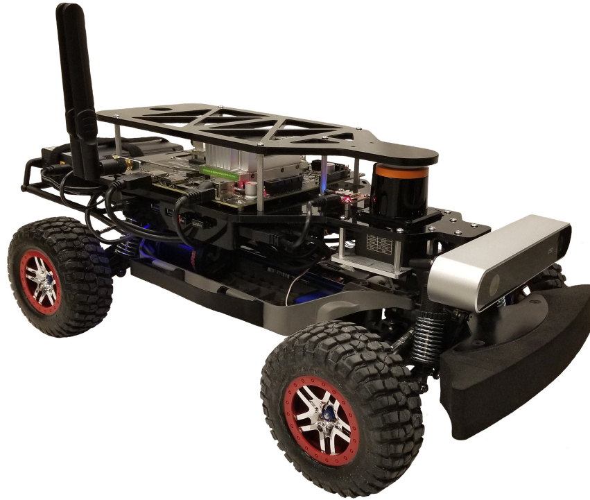
Figure 5.3: The 1/10 th scale autonomous rover used in real-world testing of LTV dynamic watermarking on a single autonomous vehicle.
