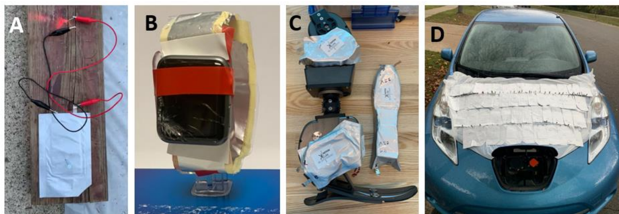
Figure 4.4: Prototypes Powered by Pouch Cells with ALPS. (A) Nail Penetration Test. (B) Health Monitoring Device (Apple Watch). (C) Robotic Prosthetic developed by Rouse Group ( https://opensourceleg.com/ ). (D) 60 pouch cells covered hood of Nissan Leaf.
