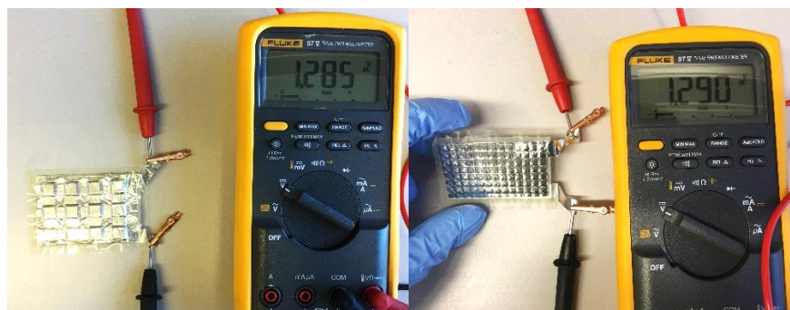
Figure S 15 The voltage generated by Zn/PZB-931/ \gamma -MnO 2 battery with different shapes. No short-circuits are observed after plastic deformation leading to corrugations.
