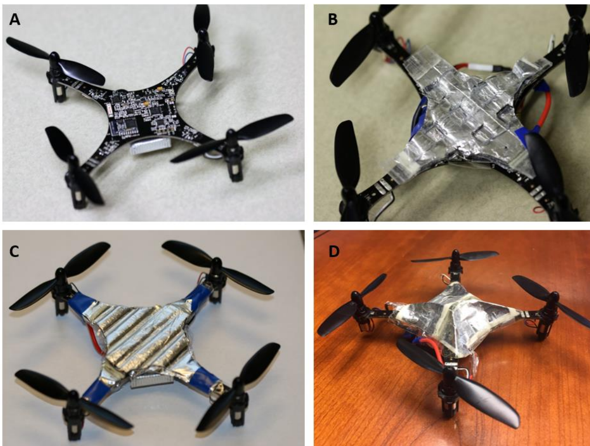
Figure 2.5 (A) Tested UAV without cover. (B, C, D) Three different designs of corrugated Zn/ \gamma -MnO 2 battery pack as a replacement for the original device cover to supplement main power source of UAVs. All modified drone models with Zn/PZB-931/MnO 2 structural batteries installed were demonstrated to successfully take off even under low ambient temperature.
