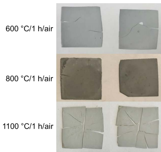
Figure D.18. Optical images of \sim 200\ \mu\text{m} ZTA films (composition D ) sintered at 1500\ \text{°C}/5\ \text{h}/\text{N}_2/\text{H}_2 , 2.5\ \text{°C}/\text{min} with different binder burnout temperatures and BN insulation.
