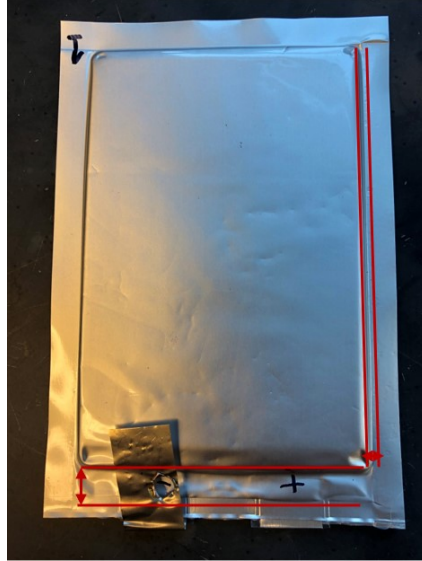
Figure 5.2: Headspace measurement for the pouch cell. The red lines indicate the widths of headspace areas. V_{h,0} can be estimated using the measured headspace area and the cell thickness. This pouch cell's headspace volume is estimated to be 13.5% of total cell volume.
