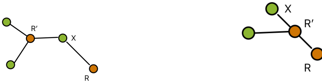
Figure B.3: Figure showing the placement of the Steiner node R' for the Zone 1 and Zone 2 recursion. The nodes in orange are Steiner nodes and the nodes in green come from the data set V .
