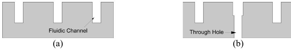
Fig. A.5: Fabrication steps of the silicon fluidic dies (a) Front-side DRIE. (b) Back-side DRIE.
