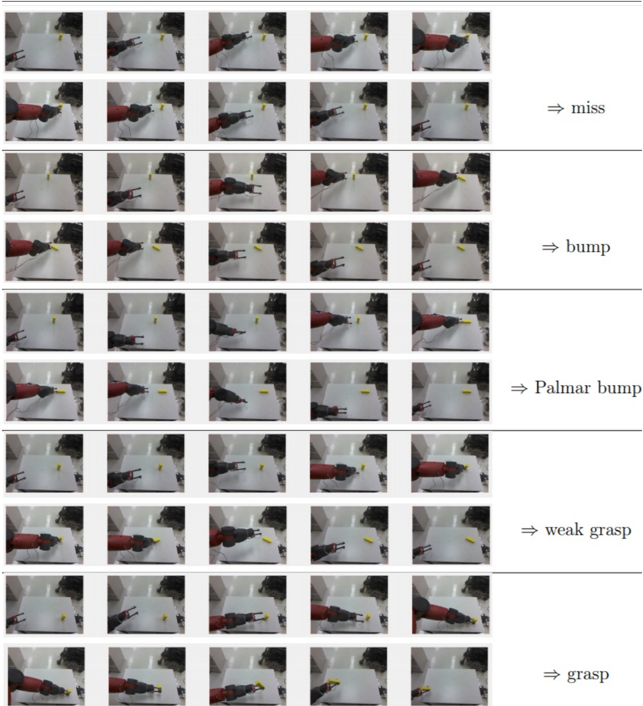
Figure 6.1: The agent’s RGB percepts during attempted grasp trajectories. Images for the forward portion toward n_f are shown in the first of each pair of rows, and images for the portion to return to n_h are shown in the second rows. Images for some nodes in the middle of trajectories with more than five nodes have been omitted. The agent classifies the result of the grasp attempt by observing the state of the target object during the trajectory. In all cases but miss , there is a substantial change between the first and last observations, and the trajectory is a successful reach. In all other cases these observations should be significantly different, and the reach component of the grasp was successful. Further classification depends on the state throughout the return trajectory and whether the Palmar reflex was activated, as discussed in section 6.1.1. Only the result of the final example is considered to be a successful grasp.
