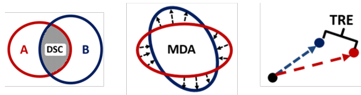
Figure 2.1. Visual representation of the three registration evaluation metrics where blue represents the ground truth and red represents DIR prediction. Abbreviations: Dice similarity coefficient (DSC), Mean Distance to Agreement (MDA), Target Registration Error (TRE).
