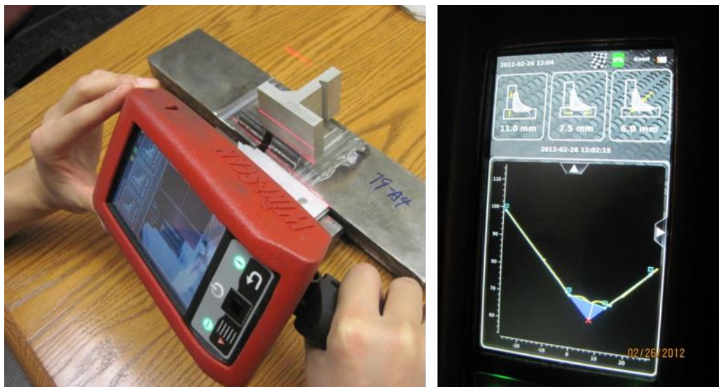
Figure 2.16: Laser scan device for weld profile and weld size determination
