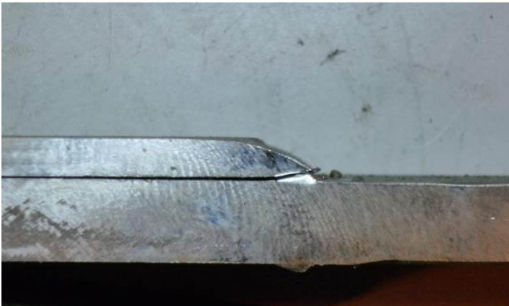
Figure 1.4: Typical weld throat failure plane observed on transverse shear specimen
