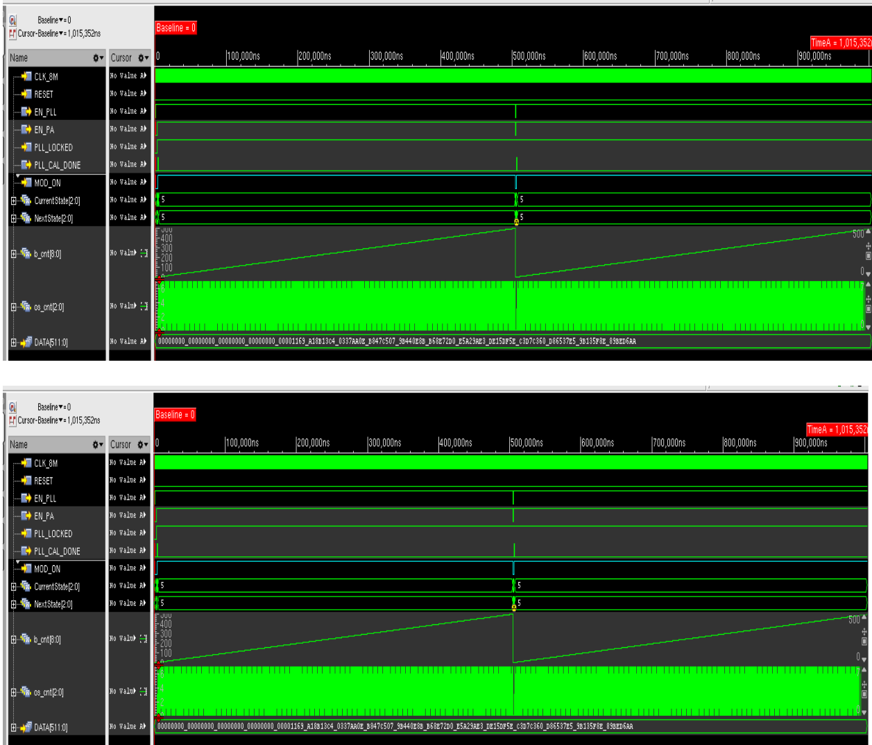
Figure 5.13 FSM timing diagram for debugging mode.
