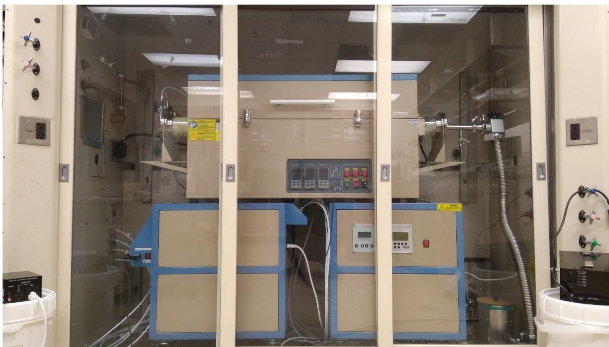
Figure 3.1 CVD equipment for MoS 2 growth, mainly consisting of the three-zone heating furnace (top), the gas control system (bottom left) and the turbo pump station (bottom right).
