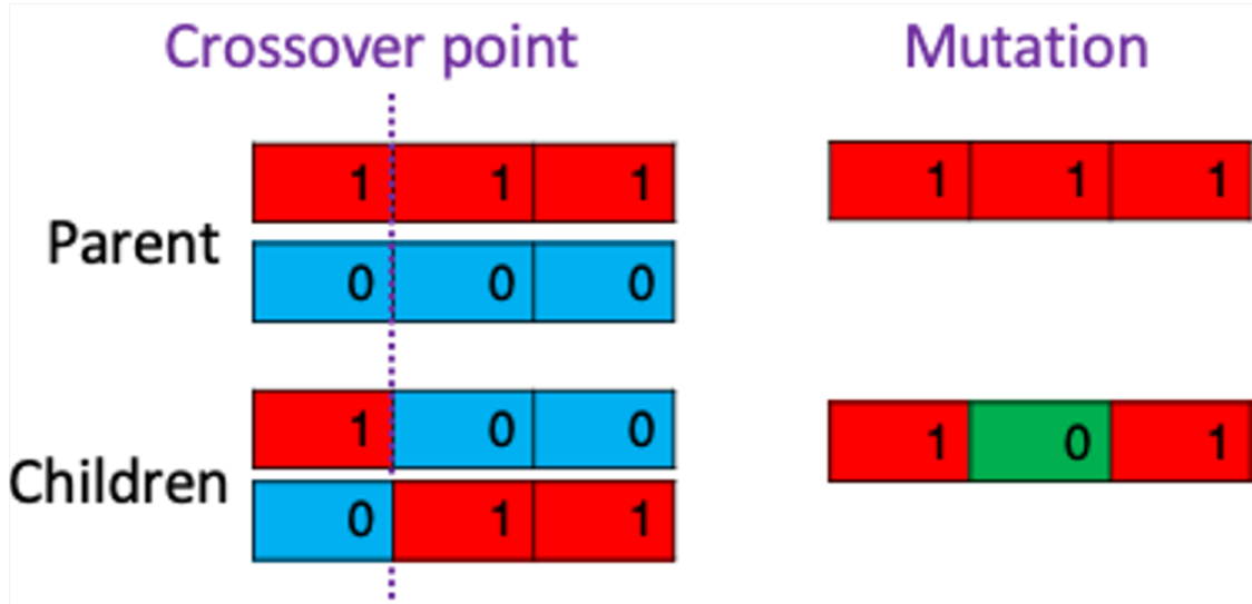
Figure 3.8: Illustration of crossover and mutation operations in the genetic algorithm.
