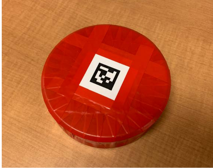
Figure 3-7. The steel drop weight used in this study featuring a red color and an AprilTag attached to both the top and bottom surfaces.
