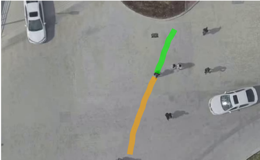
Figure 1.1: A road user in the DUT trajectory dataset. Three seconds of observed positions are shown as a solid green line. The following five seconds of positions are shown as a solid orange line.
