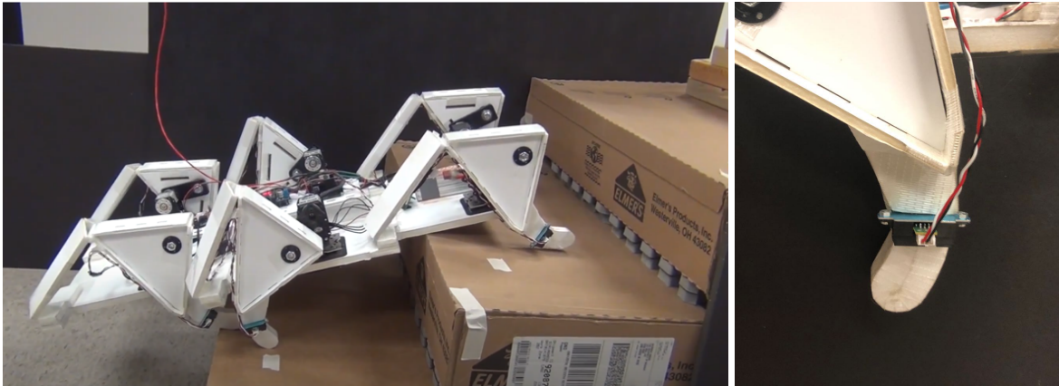
Figure 2.21: BigAnt climbing stairs (left). The distance sensor that is integrated into the BigAnt stair climbing variant (right).
