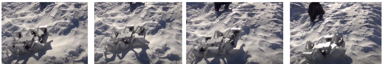
Figure 2.20: Outdoor test of the water resistant BigAnt on the wave field that is covered by 10+ cm depth of snow.
