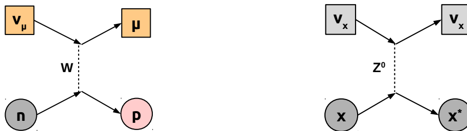
Figure 2.3: A diagram of (left) a charged-current (CC) and (right) a neutral-current (NC) interaction [8]. Note that the CC interaction reveals information about neutrino flavor based on the species of outgoing particle but the NC interaction does not.
