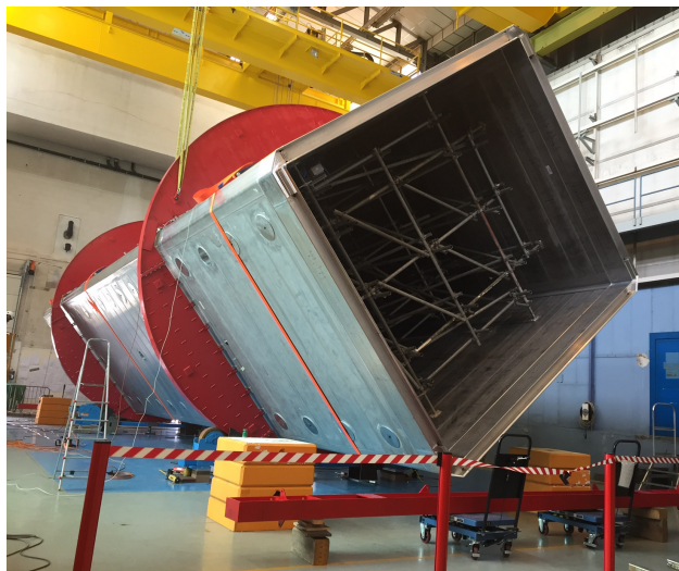
Figure 2.5: A graphic of the ICARUS detector. ICARUS consists of two modules, shown in this image (front and back).
