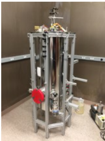
Figure 7.2: The cryostat containing the High-B setup. The magnets in the High-B setup are superconducting coil magnets and must be chilled to 4 K in order to operate.
