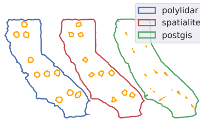
Figure 2.8: Visual comparison of different polygon extraction methods. Concave polygon output from Polylibar/CGAL (left), Spatialite (center), and PostGIS (right). Input to each algorithm was a 4000 point set sampled from the California (CA) polygon with holes per Figure 2.7a.
