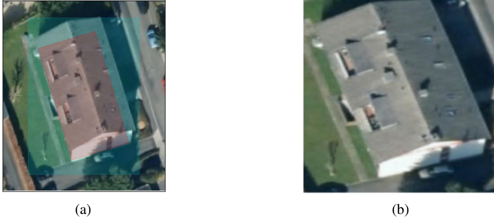
Figure 4.5: Satellite image processing. (a) Witten building outline in red shading overlaid on the satellite image. The enlarged crop area is shown in cyan shading. (b) The final generated image, resized.
