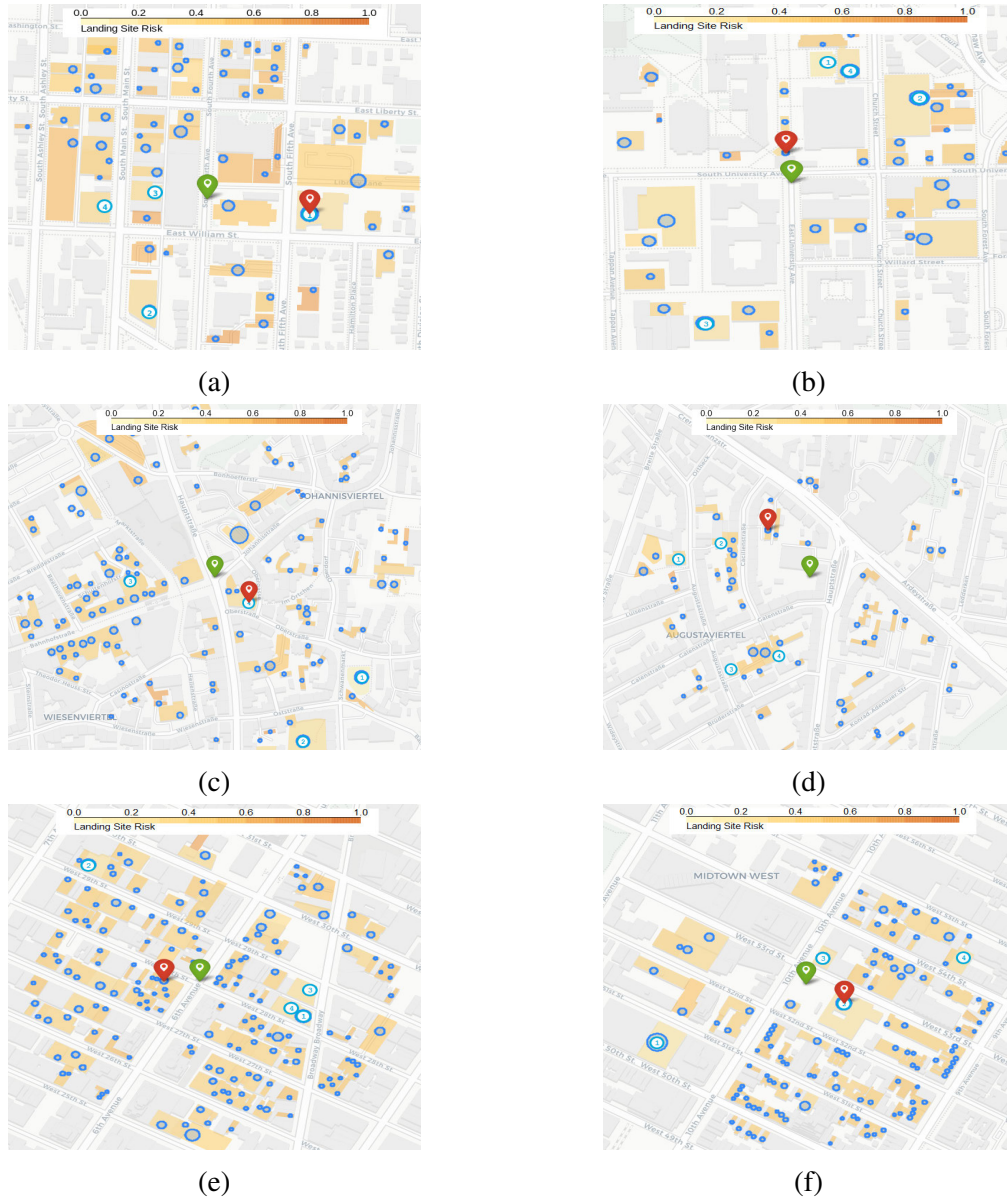
Figure 5.13: Maps of case studies for emergency landing. Maps of Ann Arbor (a,b), Witten (c,d), and New York (e, f). Failure position of the UAS is indicated by the green marker. Landing site risk is colorized from low (yellow) to high (dark orange) risk, with associated touchdown sites marked as blue circles. The lowest risk landing sites are ranked and marked with blue numbered icons. Our planner’s chosen landing site is marked in red which trades off landing site and path risk. Maps from ©OpenStreetMap contributors and ©CARTO. License: Open Database License: https://www.openstreetmap.org/copyright
