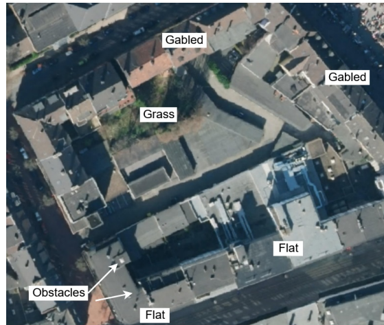
Figure 5.3: Satellite image of an urban environment with multiple flat roof landing sites. Select roof shapes and obstacles are labeled.
