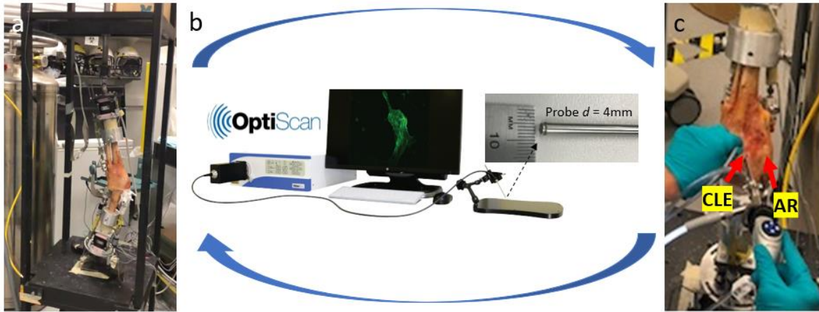
Figure 3.2 Images of the apparatus used for impulsive fatigue loading of ACL while confocal laser endomicroscopy (CLE) was used to detect changes in the ACL before, during and after the loading regimen. Changes in fluorescence were monitored approximately every 33 cycles up to 100 cycles. a) Mechanical loading device with inverted cadaver leg at an initial angle of 15° flexion generates material fatigue in the ACL after repeated pivot jump landing maneuvers. b) CLE set up with the base unit, display monitor and handheld probe attached to the base unit via a flexible waterproof cable. c) Dual probe insertion (arthroscope (AR) and CLE) through two ports located medial and lateral to the patellar tendon in order to access the proximal and distal ACL for internal joint visualization and navigation with AR and autofluorescence imaging with the CLE.
