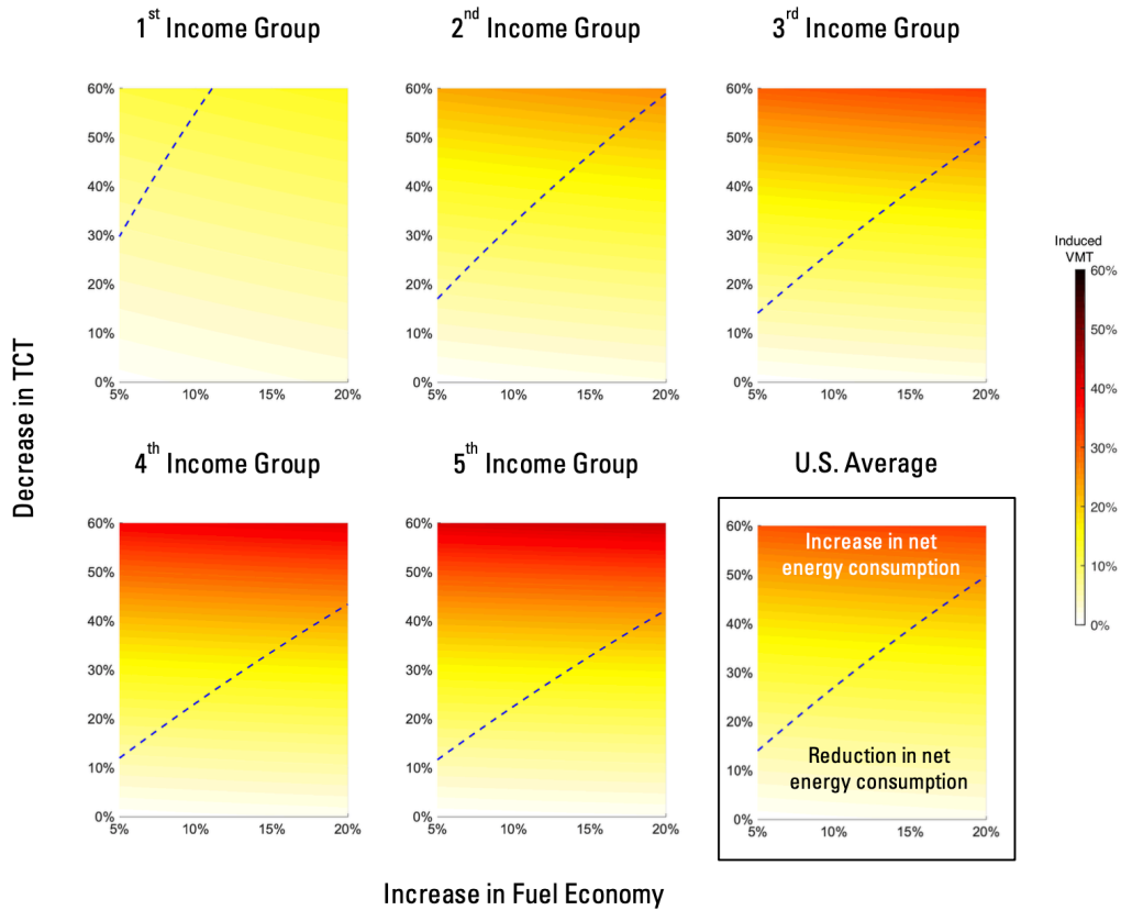
Figure A-3. Heat maps of induced travel using Model 4. All points above dashed curves are characterized by backfire in net energy consumption.
