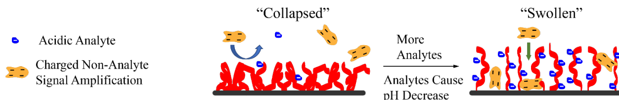
Figure 1.6. Generalized mechanism for the swelling or collapse of smart polymer brushes to amplify small molecule signals, based off of the experimental design in [92]. The analyte binds to the polymer brushes, causing signal as its charge gets near the surface. But because it is acidic, it also causes the polymer to swell. This not only allows more analyte close to the surface, increasing signal, but it also allows more charged molecules non-specifically to the surface causing signal amplification. When the analyte is not present, the collapsed polymer brush does not allow any non-analytes to the surface. Figures not drawn to scale.
