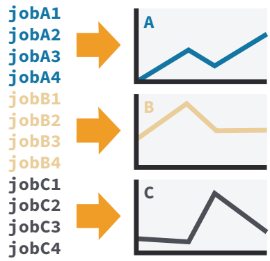
Figure 6.2: Aggregation, groups, and bundling allow users to build complex workflows. The features are orthogonal, and can be used in any combination. Aggregation enables one operation or group to act on multiple jobs. Groups allow users to combine multiple operations into one, with dependencies among operations resolved at run time. Bundling helps users efficiently leverage HPC schedulers by submitting multiple commands in the same script, to be executed in serial or parallel.
