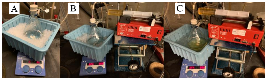
A) Reaction flask set-up after addition of starting material (1) and toluene; B) reaction solution before the n BuLi addition; C) reaction solution during the n BuLi addition
