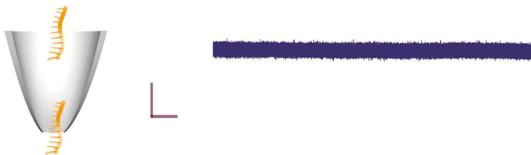
Figure S16. Sensing of miRNA without AuNP probes. The current-time trace of miR-141-3p (10 nM) nanopore sensing (Scale bar: vertical 50 pA, horizontal 5 s). The translocation experiments were performed in 50 mM KCl, 10 mM Tris-EDTA, and at a voltage of -600 mV. The current-time trace is recorded at a 1MHz sampling rate and filtered using a low-pass Bessel filter with a cut-off frequency of 100 kHz. There are no observable translocations.
