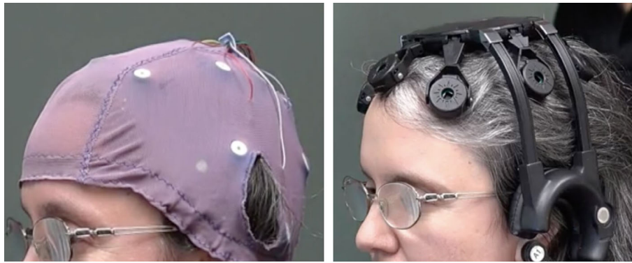
Figure 3. Photo comparing brain-computer interface headgear types: gel electrode cap (left) and dry electrode headset (right).
