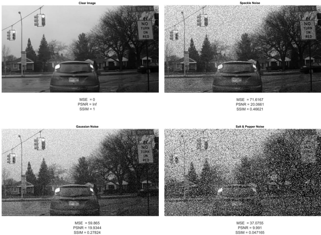
Figure 2-10: When comparing an image to itself (top left), MSE = 0, PSNR = infinity, and SSIM = 1, as expected. MSE and PSNR scores, however, are not aligned to human perception of image quality, unlike SSIM.
