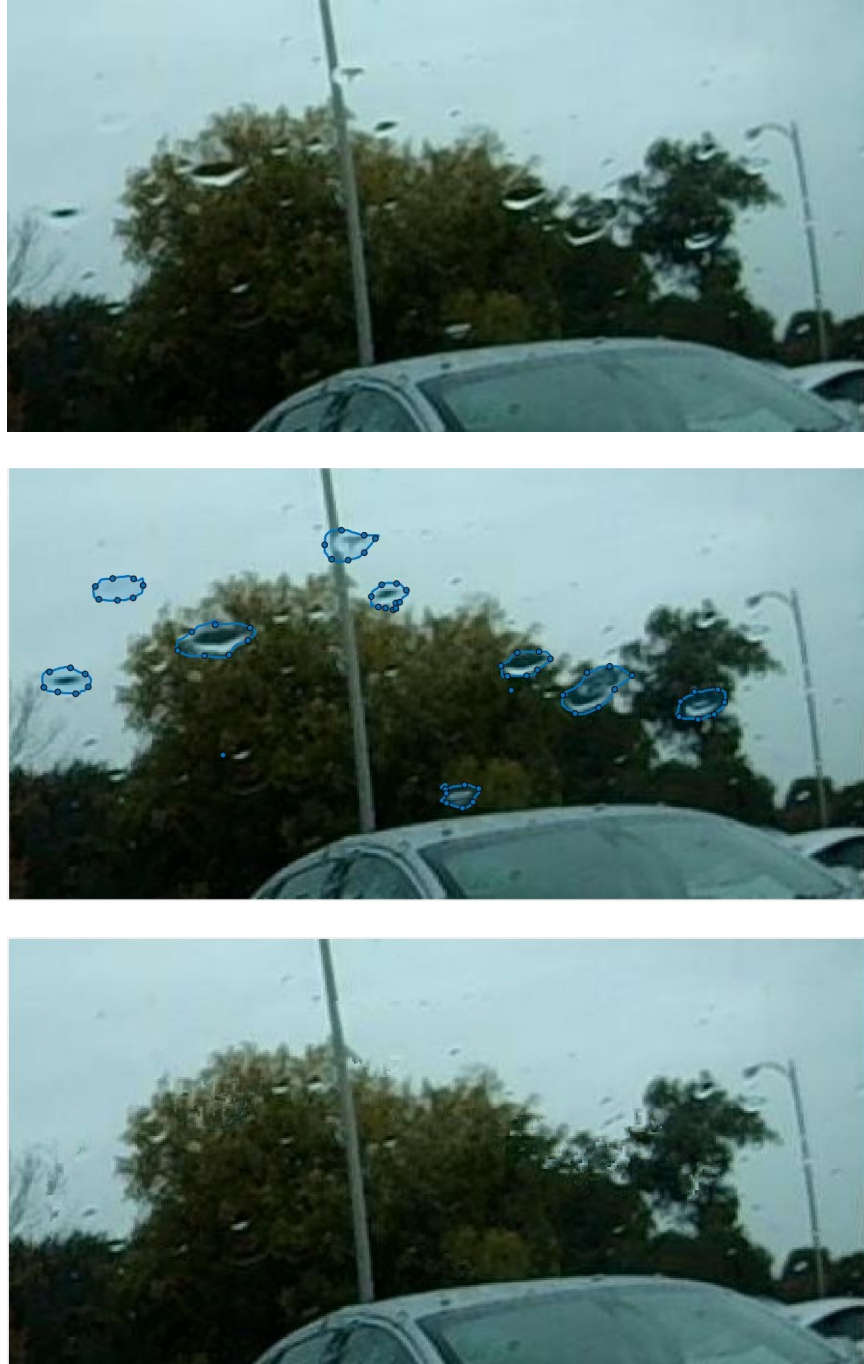
Figure 2-7: For a rainy image (top), the raindrop detection algorithm identifies areas of a raindrop in the image (middle). Image inpainting is then used to restore the image, effectively removing rain from the image (bottom)
