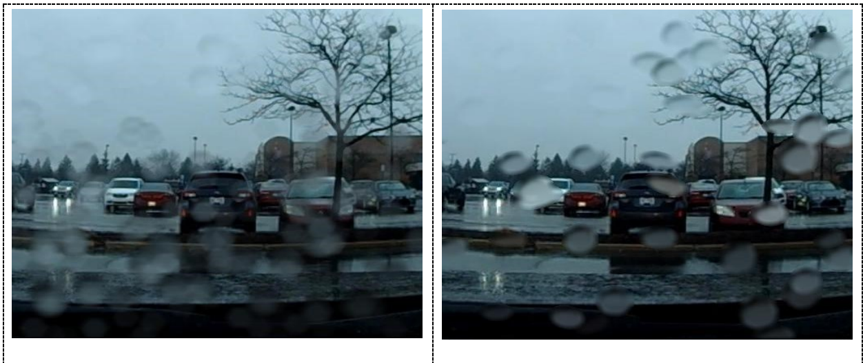
Figure 6-14: Images with raindrops that were generated by the ray-tracing method (left) and our method (right). Our model generates raindrops with more varieties in size, shape, and orientation compared to the ray-tracing model. The transparency levels in our generated raindrops are closer to that of real drops and are generally lower than that of raindrops generated by the ray-tracing model.
