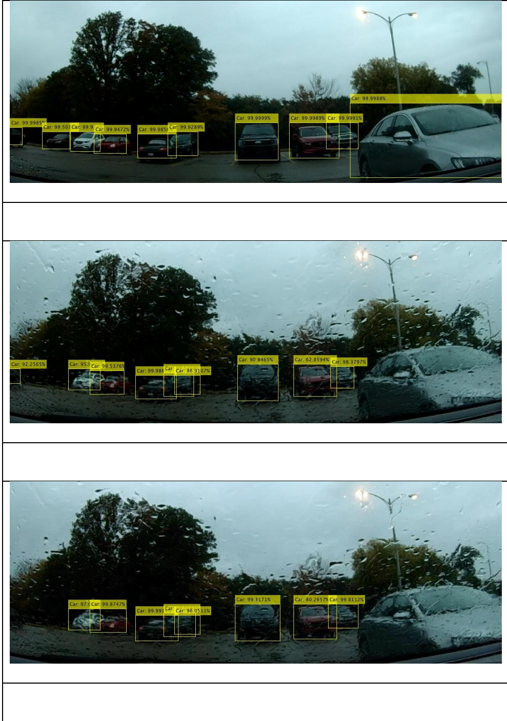
Figure 7-5: An example of the output of the YOLOv3 detector that was trained in stage 2 using clear, rained, and de-rained datasets. The objects are identified with a bounding box, with a class tag and detection confidence level shown for each object. Not much rain content was removed by the de-raining algorithm and no detection performance improvement in the de-rained image compared to the rained one.
