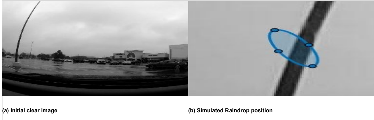
Figure 6-4: Starting with a clear image frame (a), the simulator generates arbitrary values for simulated raindrop location, size, and orientation (b).
