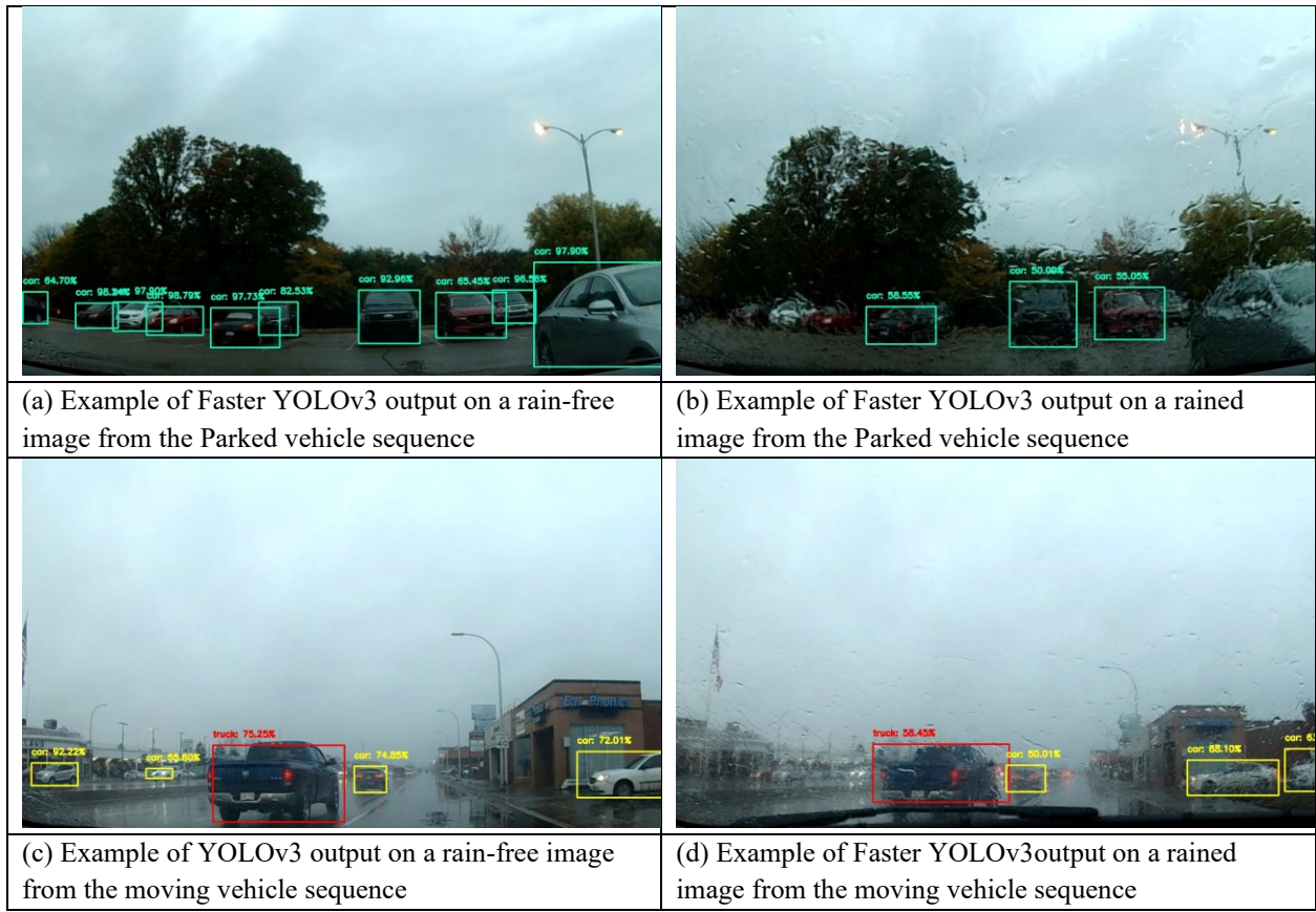
Figure 5-11: More objects are detected using YOLOv3 in the clear image (a and c) than in the rained image (b and d). For detected objects, detection confidence in the rained images is lower than that in clear ones.
