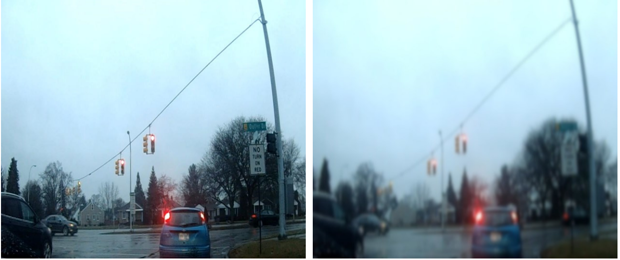
Figure 2-1: The blurred image (right) is created by applying a blurring effect using a 2D Gaussian filter with a standard deviation of 4.5 to the original image (left). Sharp edges are smoothed out, which can be noticed on the traffic sign text becoming unreadable in the blurred image.
