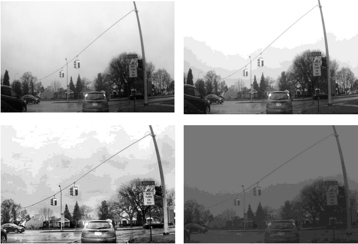
Figure 2-5: Some techniques to adjust the brightness of the image (top left) include adding a fixed bias (top right), using histogram equalization (bottom left), and intensity remapping (bottom right).
