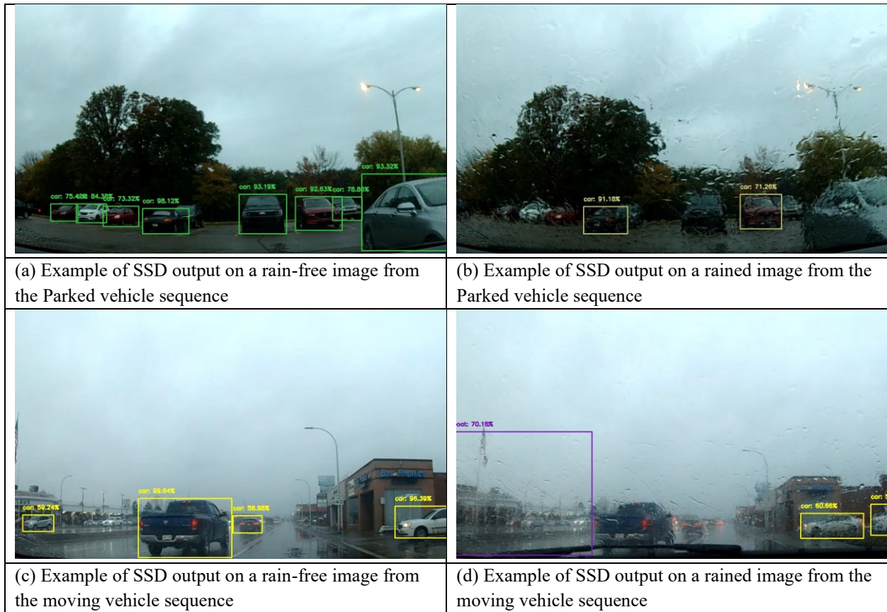
Figure 5-7: More objects are detected using SSD in the clear image (a and c) than in the rained image (b and d). Moreover, some misclassifications are found in the rained image (d). For detected objects, detection confidence in the rained images is lower than that in the clear images.
