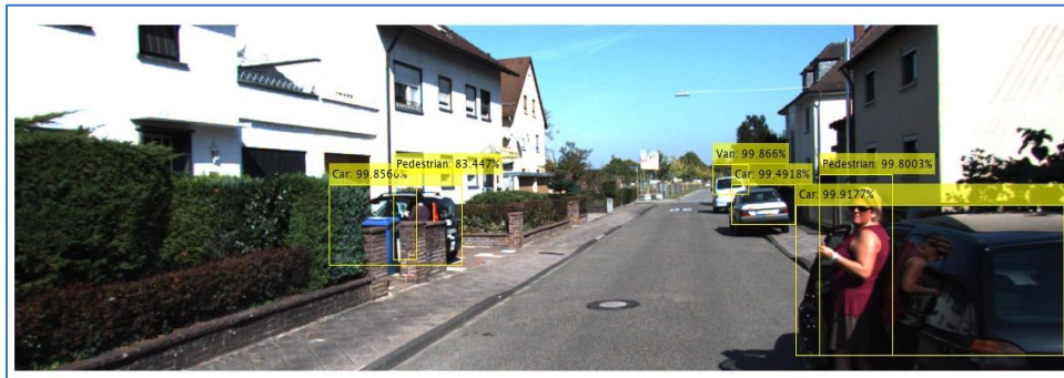
Figure 7-4: An example of the output of the YOLOv3 detector that was trained in stage 1. The objects are identified with a bounding box, with a class tag and detection confidence level shown for each object.
