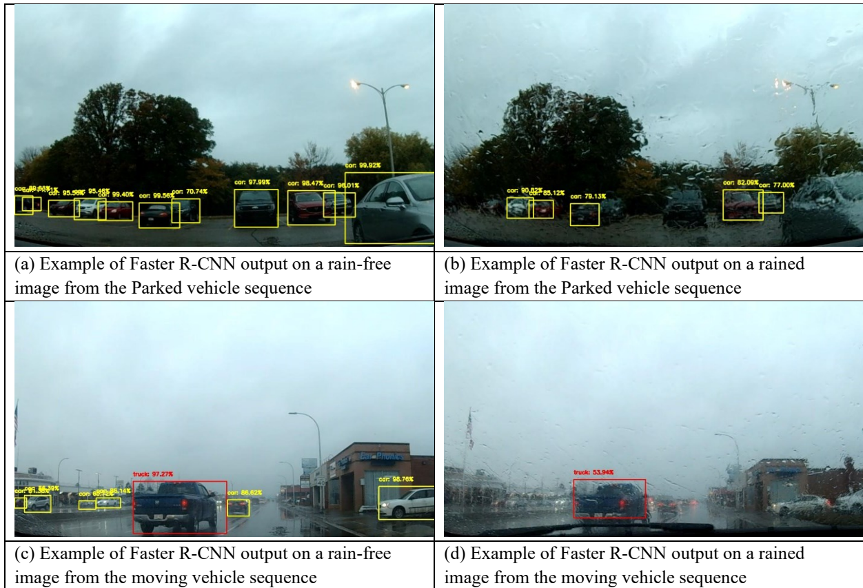
Figure 5-9: More objects are detected using Faster R-CNN in the clear image (a and c) than in the rained image (b and d). For detected objects, detection confidence in the rained images is lower than that in clear ones.
