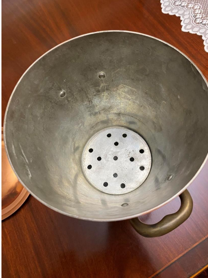
Figure 5. Replace the circular plate. Make certain it does not touch the water under it.
