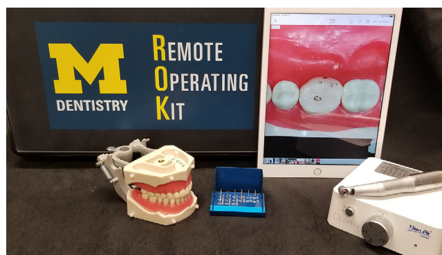
FIGURE 1 Remote Operating Kit: Columbia R861 typodont, Bien Air electric hand piece with Optima controller, diamond bur kit, iPad, carrying case
