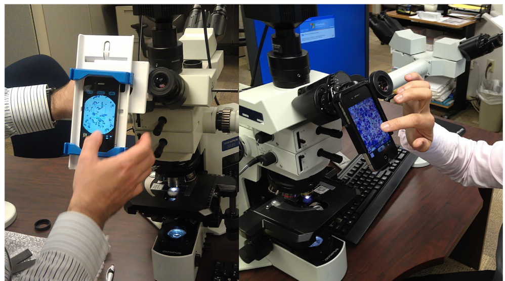
FIGURE 1 Telecytology in action with two different types of microscope adapters for cell phones. Left, Skylight adapter. Right, Magnifi adapter [Color figure can be viewed at wileyonlinelibrary.com ]
