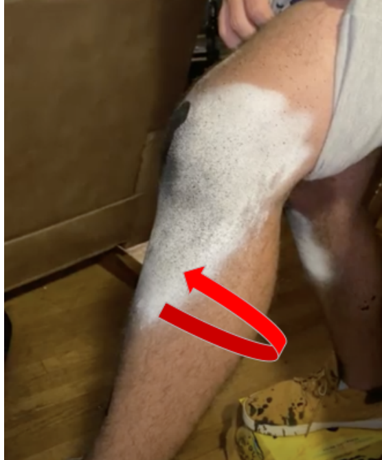
Figure 12: Applied knee speckling and direction of rotation
