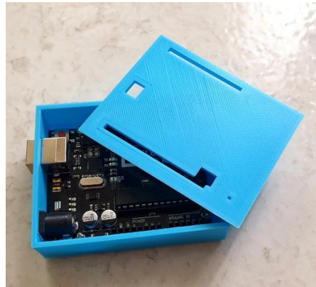
Figure 10. Image of the 3D printed enclosure. ( https://www.thingiverse.com/thing:4341737 )
