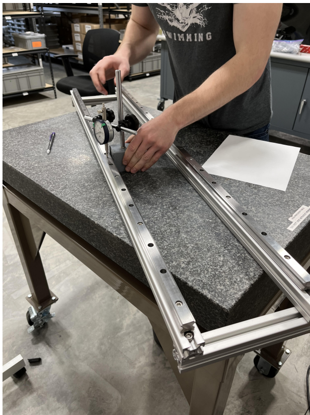
Figure 29: Carson uses a dial indicator to check for deviation in height across the rail. Note: This is an additional step that was taken and not what was described in the procedure above. In the procedure, the entire frame was upside down compared to this view.
