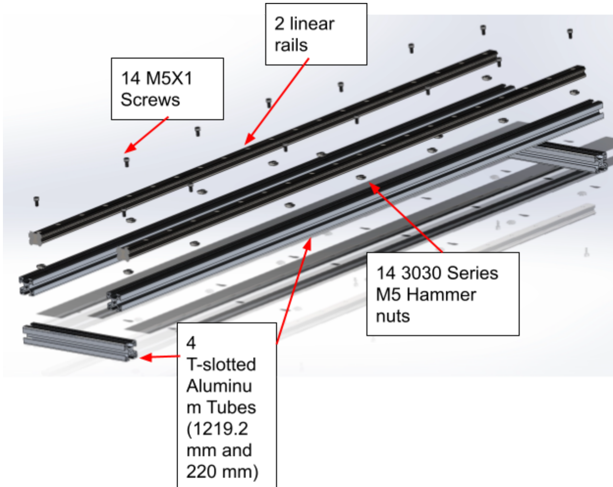
Figure 37 The diagram shows the exploded view for the frame assembly using various screws, linear rails, and t-slot aluminum extrusions.
