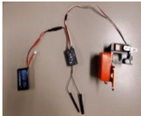
Figure 29. Depicts the pin method. On the left of the picture there is a grey U shaped slot with a pin going through the top of the U. With a push of a button that pin will be retracted dropping the fin design.
