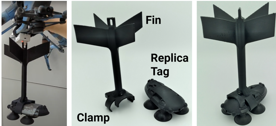
Figure 22. (Left) All three sub assemblies combined with a DJI phantom for testing. (middle and right) The final design for the fin and clamp, with a 3D printed tag.
