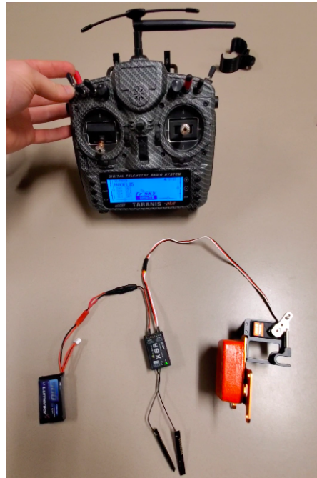
Figure 20. RC Controller (transmitter), lipo battery, receiver, and servo-motor used to power the pin release system prototyped by Ocean Alliance for their Splash Drone.
