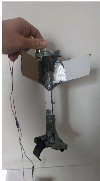
Figure 19. The fin system is attached to the electromagnet. The electromagnet is turned on and is holding up the fin system via a piece of metal attached to the top of the fins.
