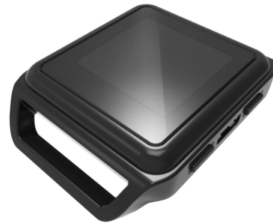
Figure 5. OPAL wearable sensor used in the Sienko Research Group's solution to detect fetal movement
