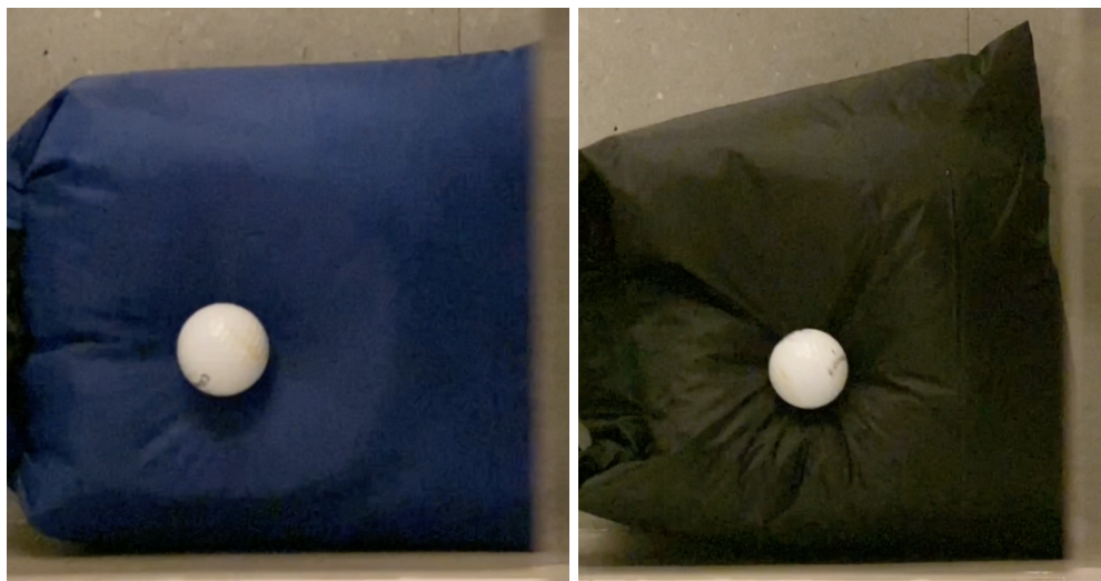
Figure 30. Dry bag bag with water and foam fill, load from 30 in height
