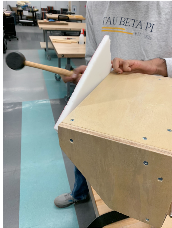
Figure 63B. We used pieces of foam between the mallet and footrest to avoid damage to the wood
