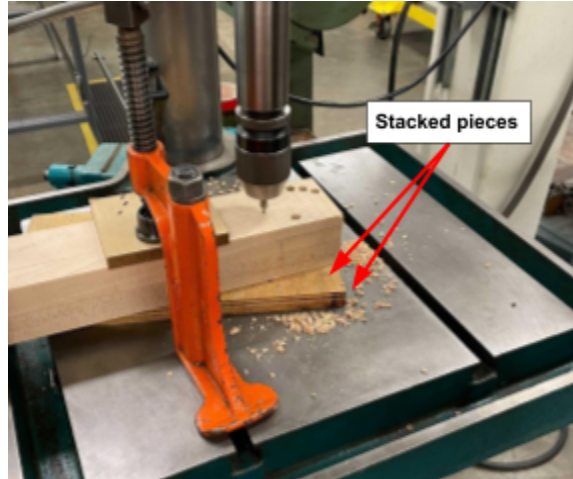
Figure 57. Match drilling example on a drill press. Both parts are identical, and used symmetrically on the device. Multiple clamps keep the parts aligned with each other and secure on the table.
