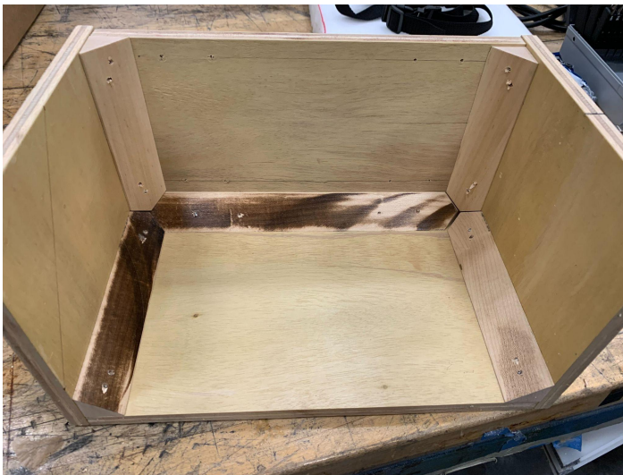
10 Assembly foot support beams to connect foot-box and seat together
