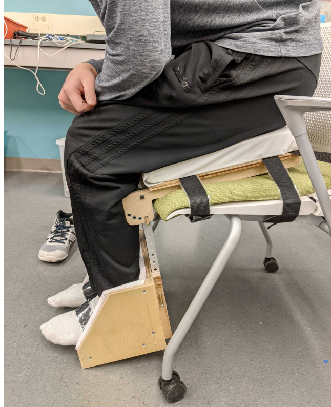
Figure 61. The device tipping when the user puts their weight onto the footrest
