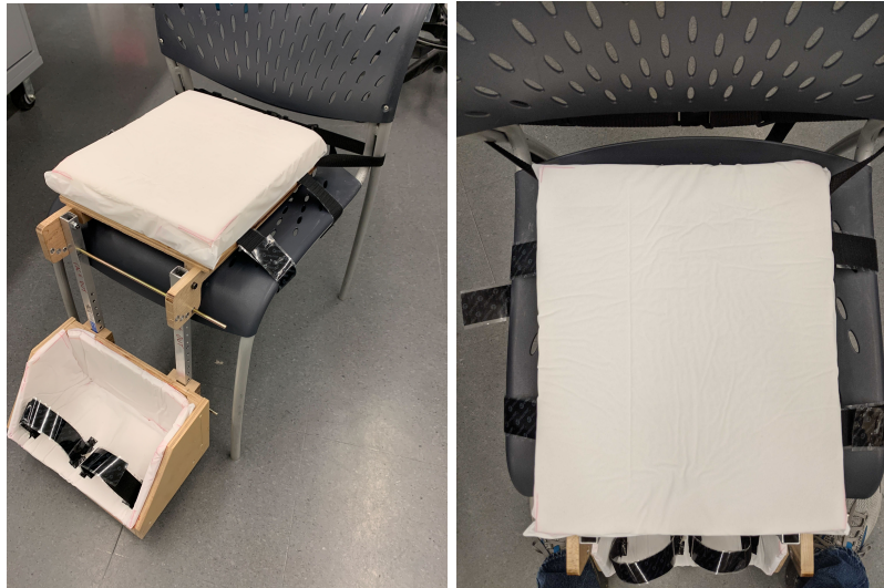
Figure 43. The foot support is strapped to a chair. The image on the right shows a top down view to make the locations of the straps clearer.
