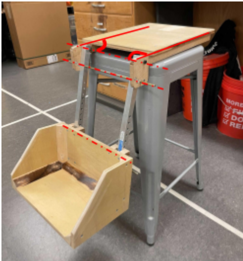
Figure 58A. Foot support adjustment alignment locations. These axes are critical to be aligned symmetrically about the midplane of the device. The distance shown at the bottom is critical (shown in 44B on the right, as the beam needs to abut against the back of the footbox as shown).
