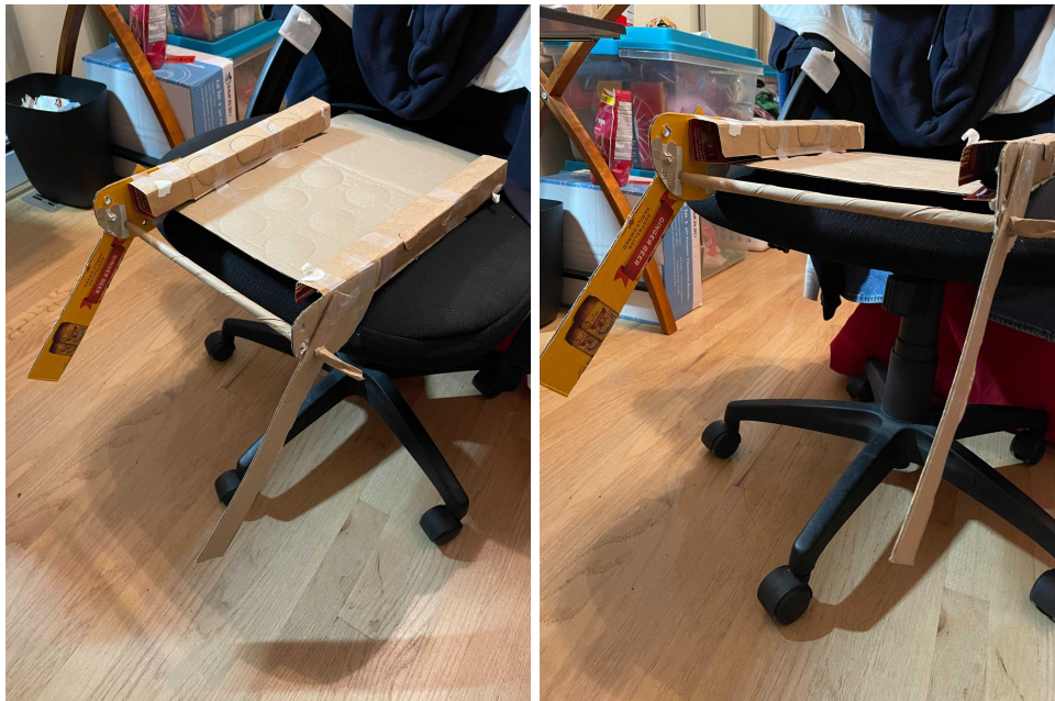
Figure 28. A full scale low fidelity prototype made from cardboard to help us understand how knee flexion would interface with the rest of our alpha concept.
