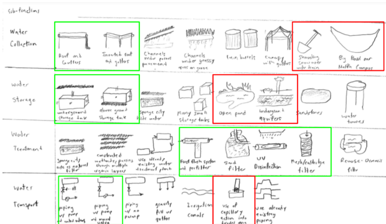
Figure 5. Our morphological chart; the green boxes indicating ideas that would work best in conjunction with our design and the red boxes indicating designs that would not be as feasible.
