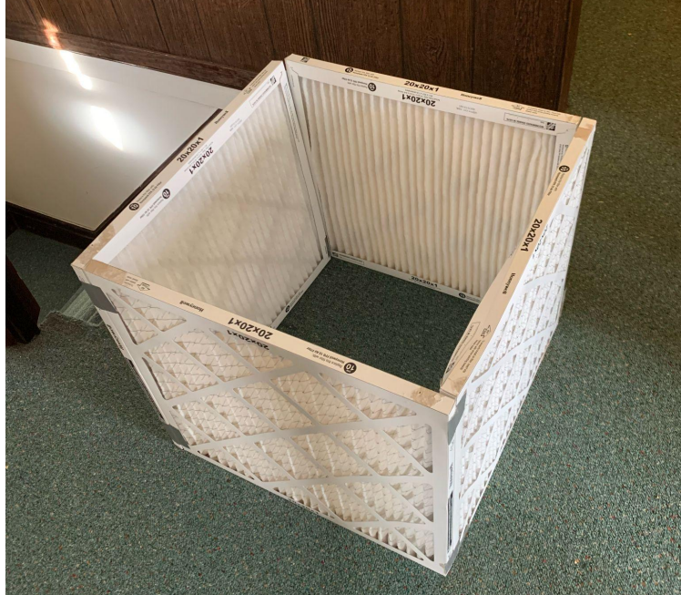
Figure 15: Filters tapes in cubic shape ready to be attached to the box fan.
