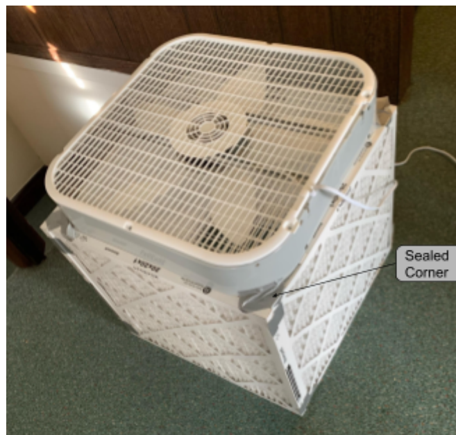
Figure 16: Sealed corner of filter and fan connection
