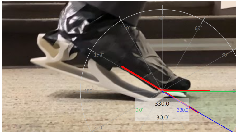
Figure 41. This is how the Moon Shoe deforms. As seen in the image, there is 30° of forefoot flexure, which is more than the required 15°.
