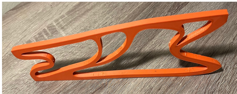
Figure 42. A sample print of the Moon Shoe. This was printed out of Nylon without the Kevlar reinforcement.
