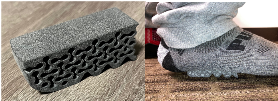
Figure 38. The TPU 88A print that we ordered (left). As seen in the deformation, it behaves as we expected and compresses when loaded (right).
