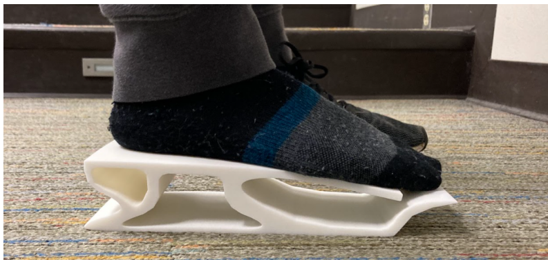
Figure 51. Deformation of the Moon Shoe prototype during midstance, there is minimal to no deformation at the heel and midfoot. The Moon Shoe is 2" loaded and unloaded.
