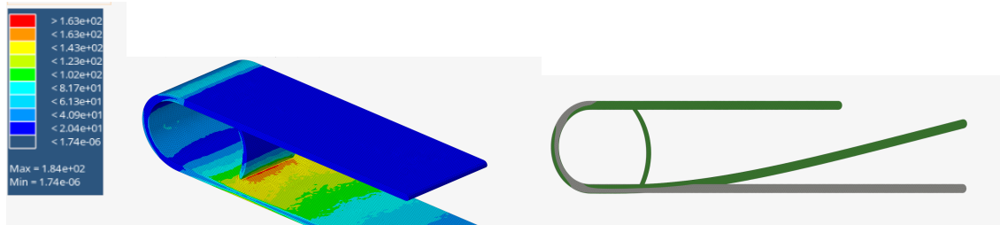
Figure 41. Here we can see how just adding one rib helps increase stress to 184 MPa (left) and decreases deformation to 45 mm (right). We can also see that the location of the major stresses shifts. Although this is an improvement, the design would still fail stresses and deformation.
