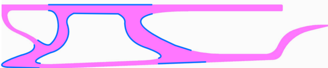
Figure 56. The blue lines show the thicker areas that could be reduced to save money and time.
