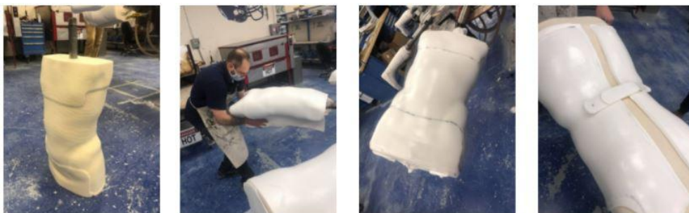
Figure 4. Pictures showing part of the current manufacturing process for TLSOs
