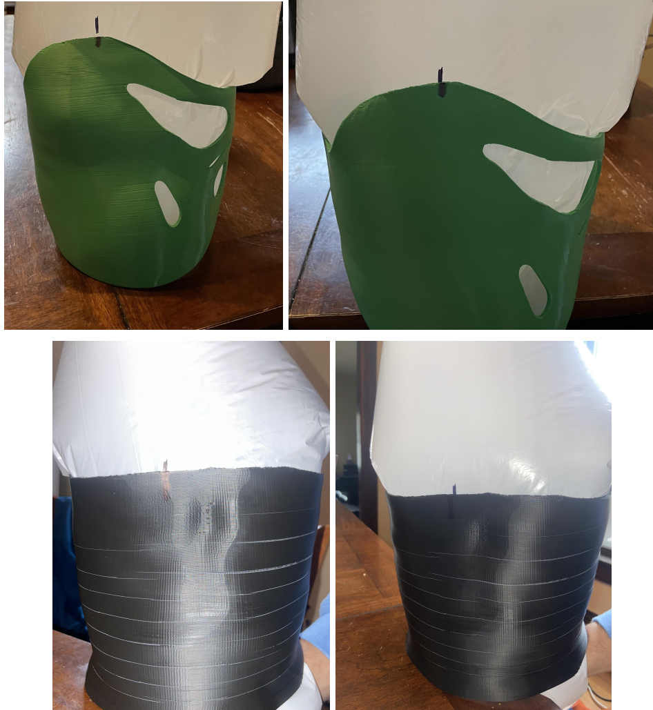
Figure 29. The photos show the relative movement of the optimized TLSO (top) and baseline TLSO (bottom) after twisting 45 degrees left of center and 45 degrees right of center and positioned back at 0 degrees.
