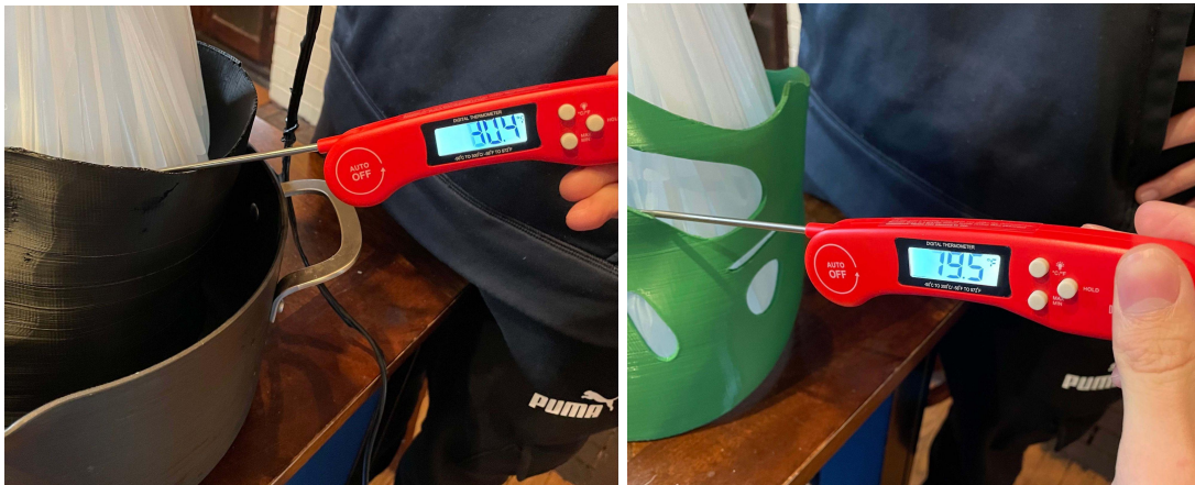
Figure 27: The steady state temperature of the TLSO was captured using a temperature probe on the surface of the skin. The resulting temperatures can be seen and were recorded: 80.4°F for the optimized TLSO and 79.5°F for the baseline TLSO.
