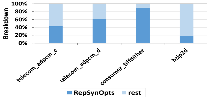
Figure 3.17: Diverse applications with -fno-if-conversion and -fno-ssa-phiopt in their synergistic optimizations. Breakdown shows their importance in each customized setting.
