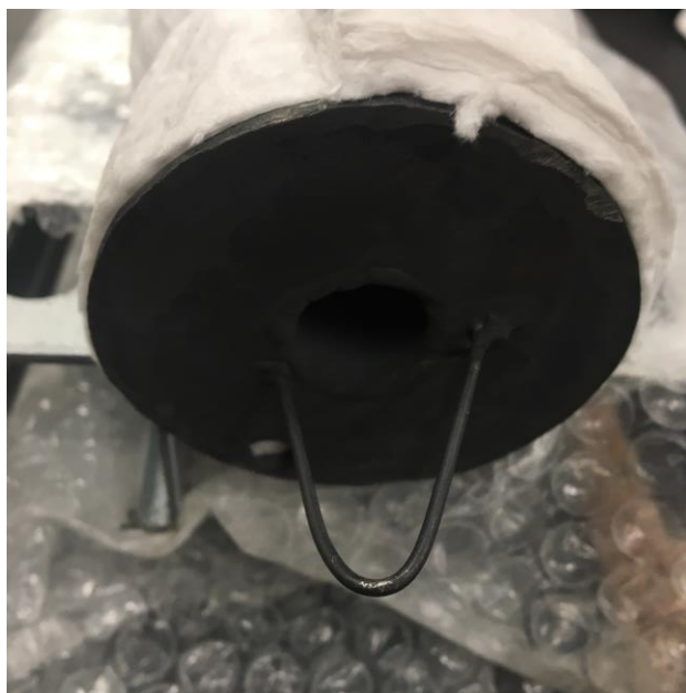
Figure 3-13 Thermal insulation holder on the outlet intrusion tube
