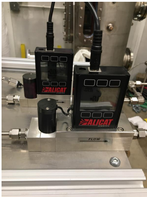
Figure 2-7 Gas mass controllers used for flow control
