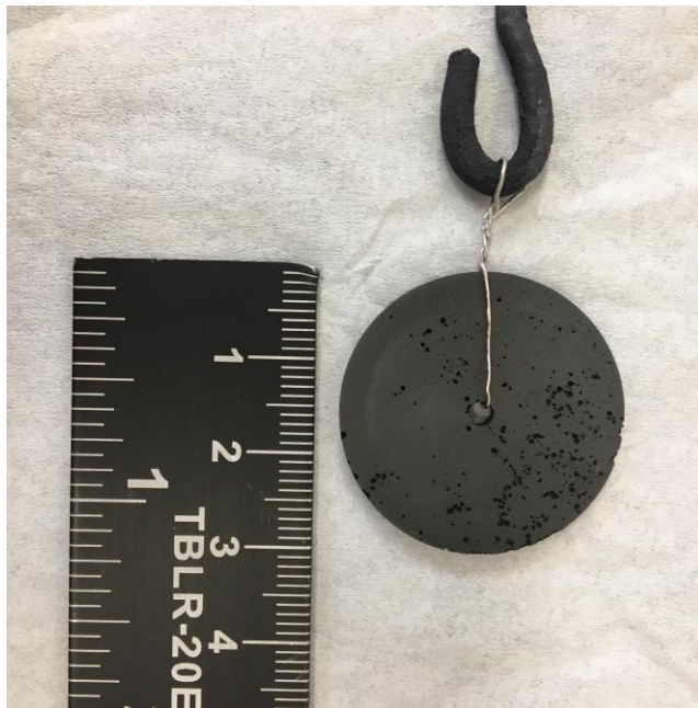
Figure 3-11 Graphite sample with local oxidization spots
