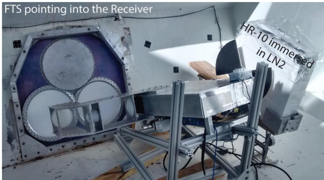
**Figure 4.1:** FTS and coupling optics set-up at the AdvACT site [55]. The FTS rests on a mount that angles such that the detectors are illuminated at normal incidence. The top image shows the set-up using a heat lamp source, and bottom shows the set-up using HR-10 Eccosorb immersed in LN<sub>2</sub> as a cold source. Preliminary data analyses showed that both sources produced around the same S/N in the measurements. The heat lamp was used for subsequent measurements due to its convenience.
