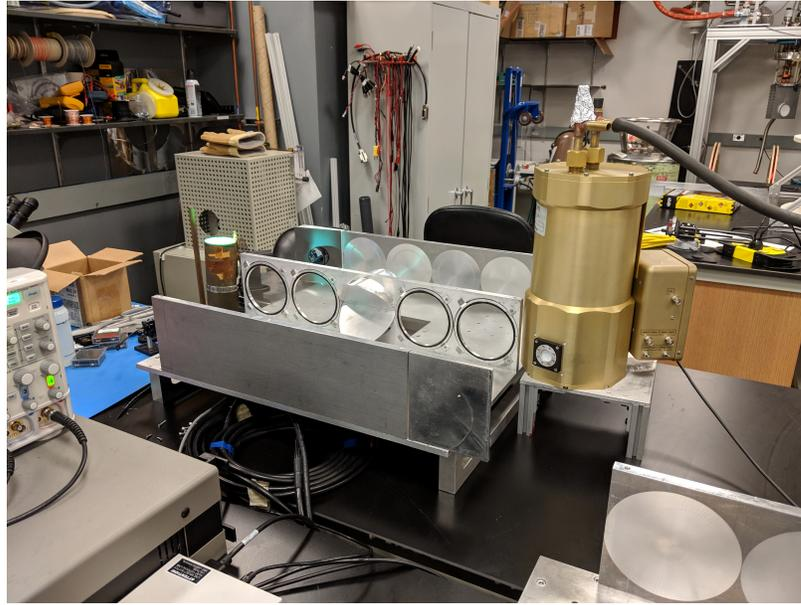
(a) A view of the single FTS measurement setup, showing the brass cryostat that houses the detector and its window entrance at the bottom of the chamber. The mercury arc lamp can be seen on the left, illuminating a transfer mirror attached to the FTS. Another transfer mirror is positioned just at the end of the beam path to direct the signal into the cryostat.
