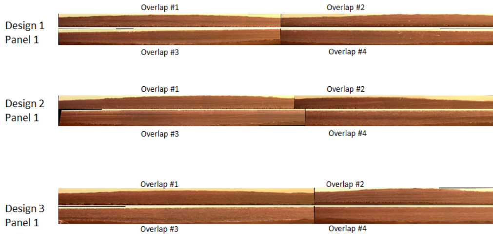
Figure 4.5: Location of microscopy specimen within the manufactured panels
