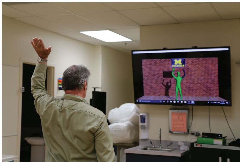
Figure 1. The set up for technology-enhanced real-time action observation therapy (TERTAOT) during a treatment session is shown. The Kinect Xbox One sensor (placed at 10 feet from the participant) captures the participant's pose data. The Jugular virtual reality system (Jugular 4.0 development) by the University of Michigan processes the Kinect pose data to create an avatar by replacing the image of the paretic limb/side of the participant with the image of the non-paretic limb/side. The Kinect application does not require preparation or calibration for the participant before each session. To begin the TERTAOT, the participant sat in a standard height chair at 10.5 feet away from the television screen and performed the TERTAOT exercises while observing the avatar performing symmetrical bilateral movements in real-time.
