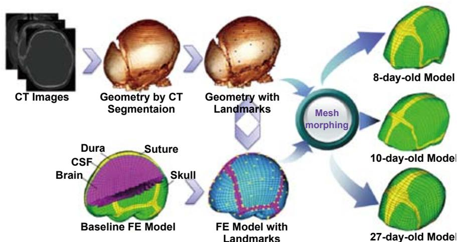
Fig. 6 Pediatric Head FE Model Construction Using Mesh Morphing Method <sup>[52, 65]</sup>
