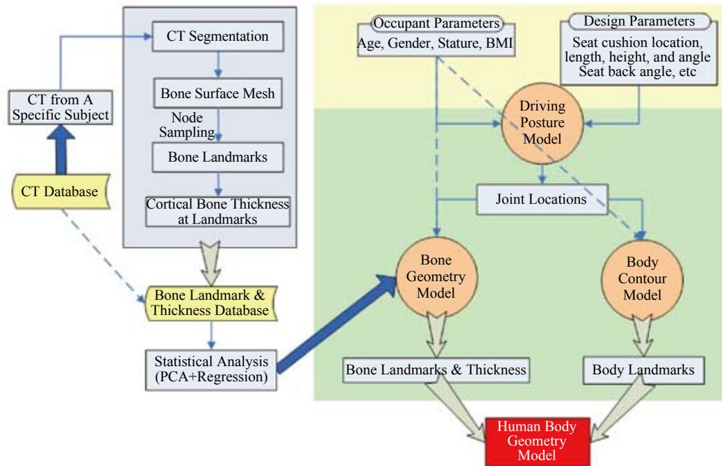
Fig. 3 Method for Developing the Statistical Human Body Geometry Model
