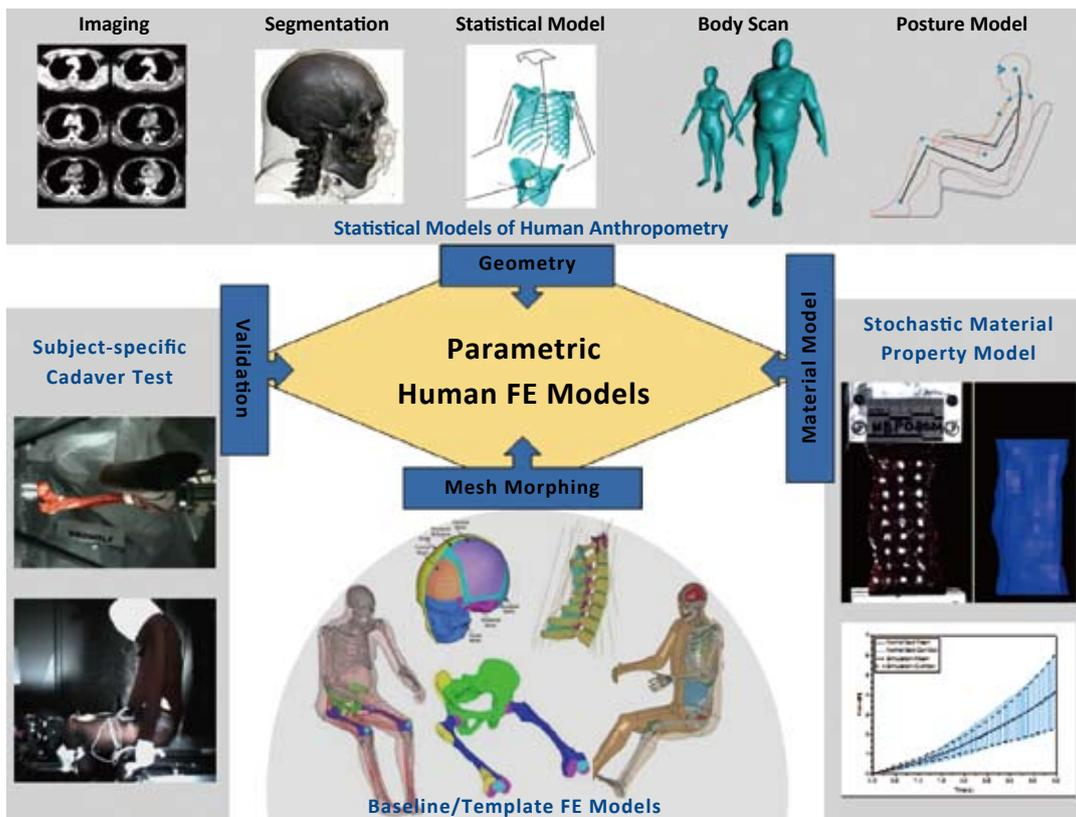
Fig. 2 Overall Technical Schematic for Developing a Parametric Whole-Body Human FE Model
