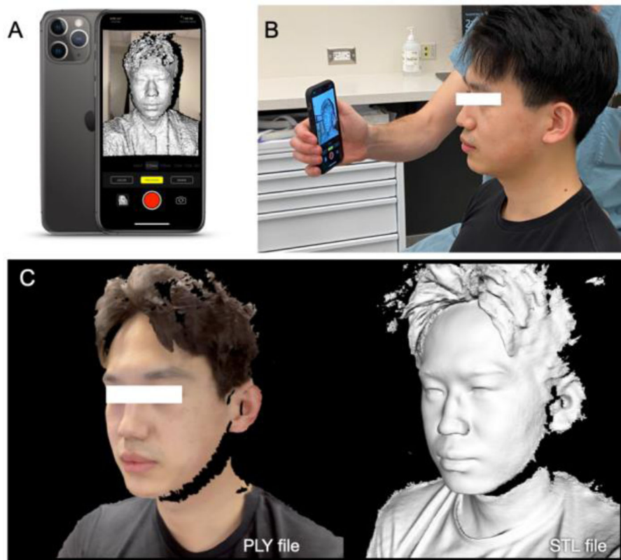
Figure 1 A, iPhone 11 pro with Heges application was used for face scan. B, Operator using iPhone to scan subject face. C, Face scan could be exported as PLY file (with color) or STL file (without color).
