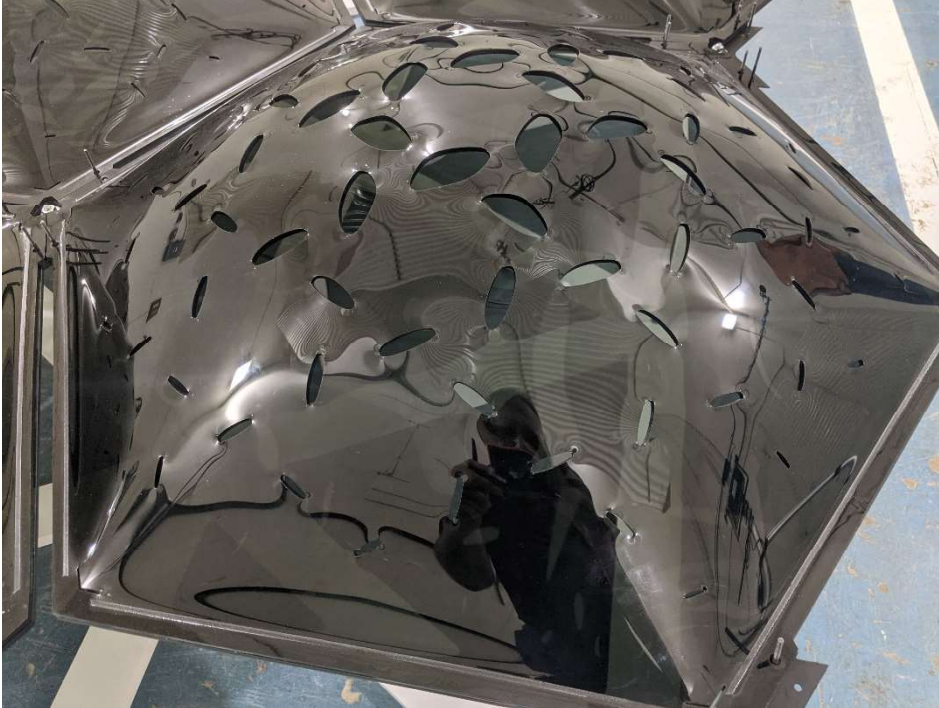
Figure 5 – Detail of curvature and perforations on some specimen glass panels
