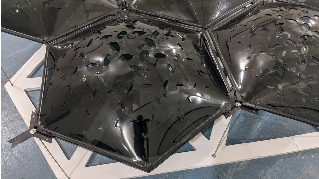
Figure 5 – Detail of curvature and perforations on some specimen glass panels
