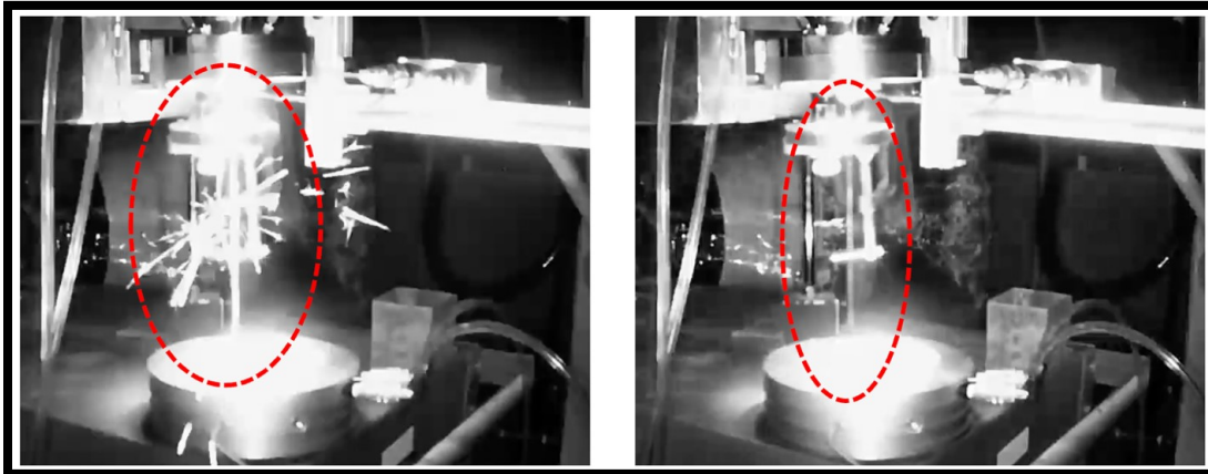
Figure 6.4b: (left) Hand baked coil at 60A of induction current clipping with the laser beam during the power test and (right) plain conical coil with a relatively larger opening bottom diameter allowing uninterrupted passage of the laser beam.
