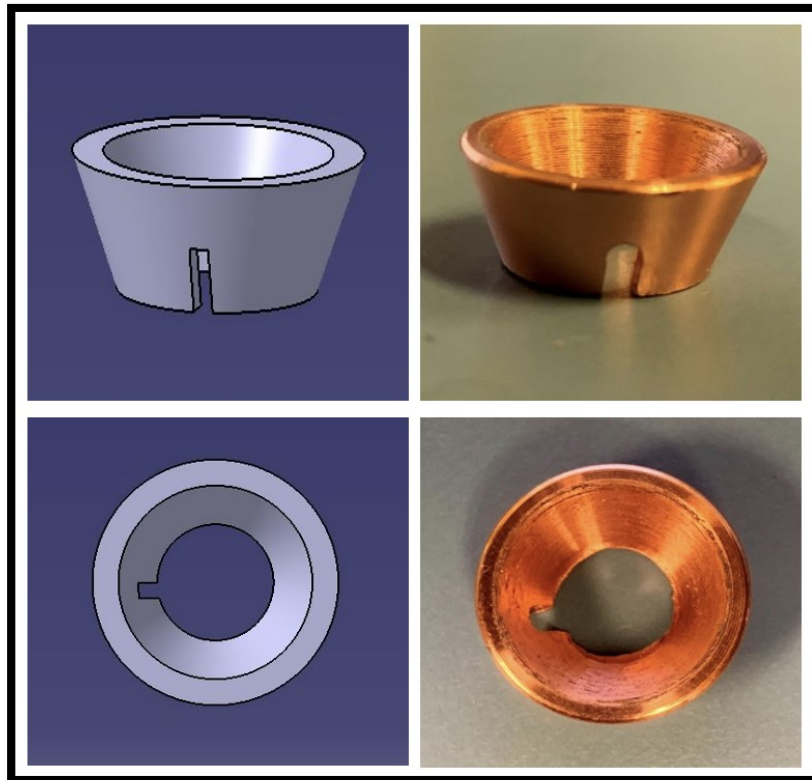
Figure 9.3: Field shaper design (left) and fabricated field shaper for ISLM coil (right)
